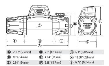
**Winch Dimensions:** 21" L x 6.3" D x 10.1" H (534mm L x 160.5mm D x 256mm H)
